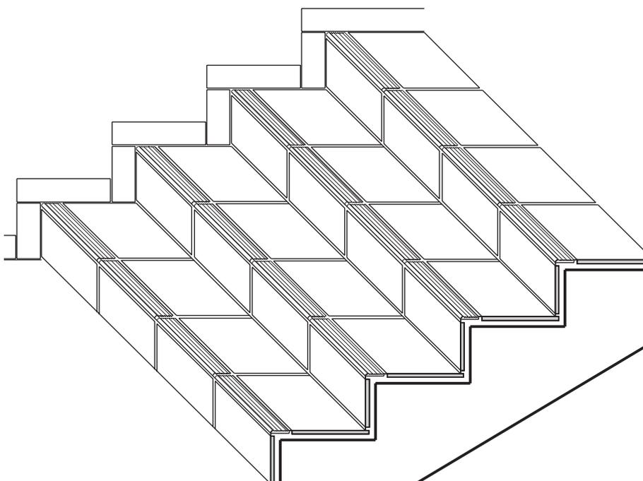
**TREPPE MIT SCHENKELPLATTEN UND HINTERLEGER, SEITLICHER ABSCHLUSS MIT SOCKELLEISTE**
